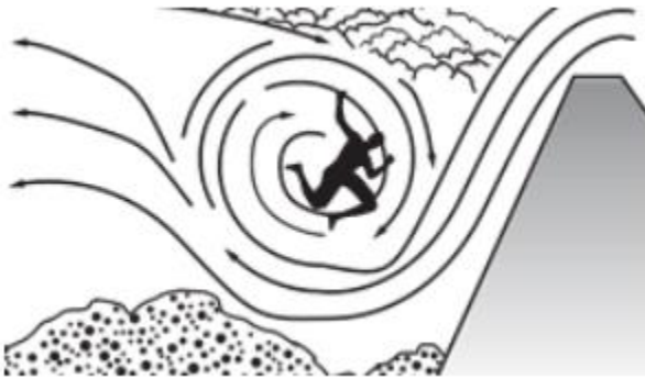
Diagram 3 - The 'washing machine effect' of being caught below a weir
